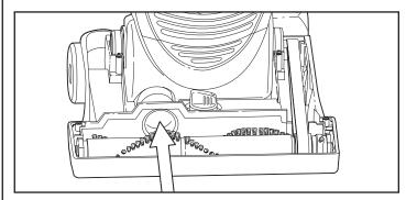
Remove the hood from the cleaner and check for a blockage in the brushroll area. Make sure the hose inlet is clear. If no blockage is found, continue to step 4.
